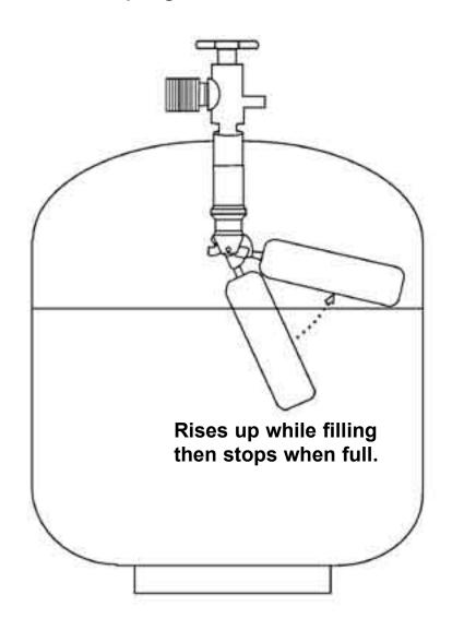
W/ANING! Do not exchange the LP Gas cylinder unless the exchange LP cylinder is equipped with an OPD. Otherwise you will lose the OPD (Overfilling Prevention Device) feature. If there is not an LP cylinder available for exchange equipped with an OPD, we recommend that you have your cylinder filled at an authorized LP gas dealer by a qualified attendant.
